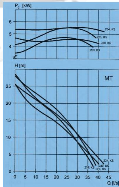
**Electro bomba sumergible FLYGT modelo 2640.180 MT**
